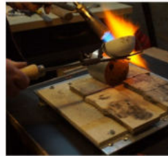
Pouring the molten silver into a two part sand mould of a case.
