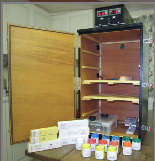
Japanese Urushi Lacquer curing cabinet. This is called a Furo in the Japanese language. Temperature and humidity required for curing changes depending on the lacquer type and pigment so a digital controller is used to set and maintain these parameters with a great deal of accuracy. (Self designed and made)
