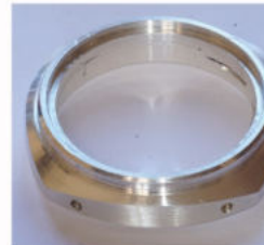
Machined silver case ready for the next drilling stage.
